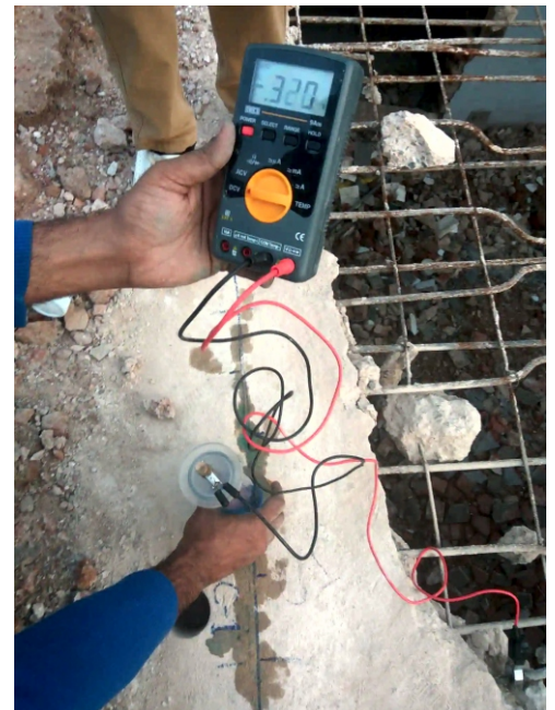
Current Measurement Using Half Cell Potential system for concrete
